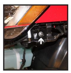
7. Using a T30 Torx, remove the three (3) screws from the driver side headlight. There are two (2) on the top side (left & middle) and one (1) on the side (right).
