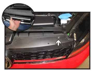
1. Using a T25 Torx, remove the two (2) screws from the top edge of the grille. There is one (1) on each side. Unsnap the grille from the vehicle and set aside.
