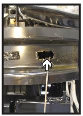
13. Using a 1-1/4" hole saw, drill an access hole on the underside of the bumper on the passenger side only (left).
