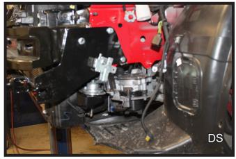
15. Prior to drilling and installing the remainder of the baseplate bolts, flatten the three (3) tabs of the horn brackets (upper left) so it will sit flat on the face of the side plate. Also it may be necessary to ream out the slot to accommodate the hardware (lower left).
