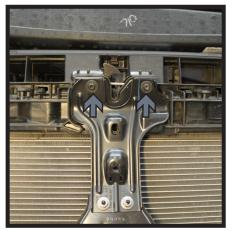
6. Using a 16MM socket, remove the eight (8) bolts from the bumper. There are four (4) on each side, two (2) on top & two (2) on bottom (white).
