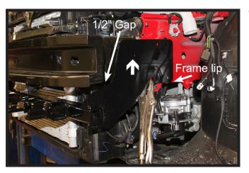
14. Position the baseplate on the vehicle so there is an approximate 1/2" gap between the baseplate and back of the bumper with the baseplate sitting on the lip of the frame. Level and clamp the baseplate.
