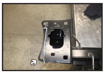
10. Temporarily reinstall the bumper. Mark the backside of the mounting flange along the cuts of the frame. Remove and trim these areas on both sides of the bumper with a reciprocating saw.
