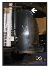
12. Trim the plastic shielding off just below the bumper on both sides of the vehicle. The shielding is not reinstalled.
