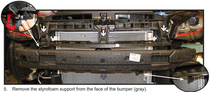
Unsnap the temperature sensor from the bottom side of the bumper and set aside.
