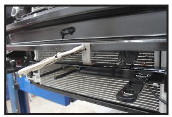
18. **Optional Breakaway:** Position the bracket in the desired location along the bottom lip of the bumper. Clamp and drill a 5/16" hole thru the bumper. Install the bracket to the vehicle with the supplied 1/4" hardware.
