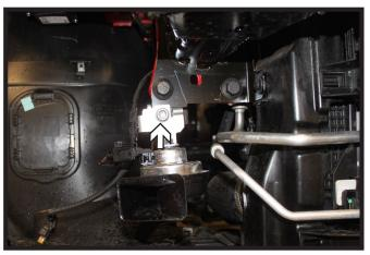
4. Using a 5/16" Allen socket or wrench, remove the screw from the horn bracket and set the horn assembly aside. Do this on both sides of the vehicle
