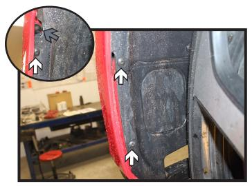
Using a T25 Torx, remove the four (4) screws from the wheel well. There are three (3) along the edge (white) and one (1) at the fascia joint (gray). Do this on both sides of the vehicle.
