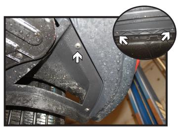
Using a T25 Torx, remove the seven (7) screws from the underside of the fascia. There are two (2) on each side in each corner and three (3) across the middle.
