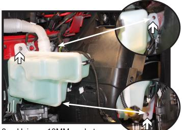
8. Using a 10MM socket, remove the three (3) nuts from the washer reservoir. Disconnect/plug all lines and set the reservoir aside.
